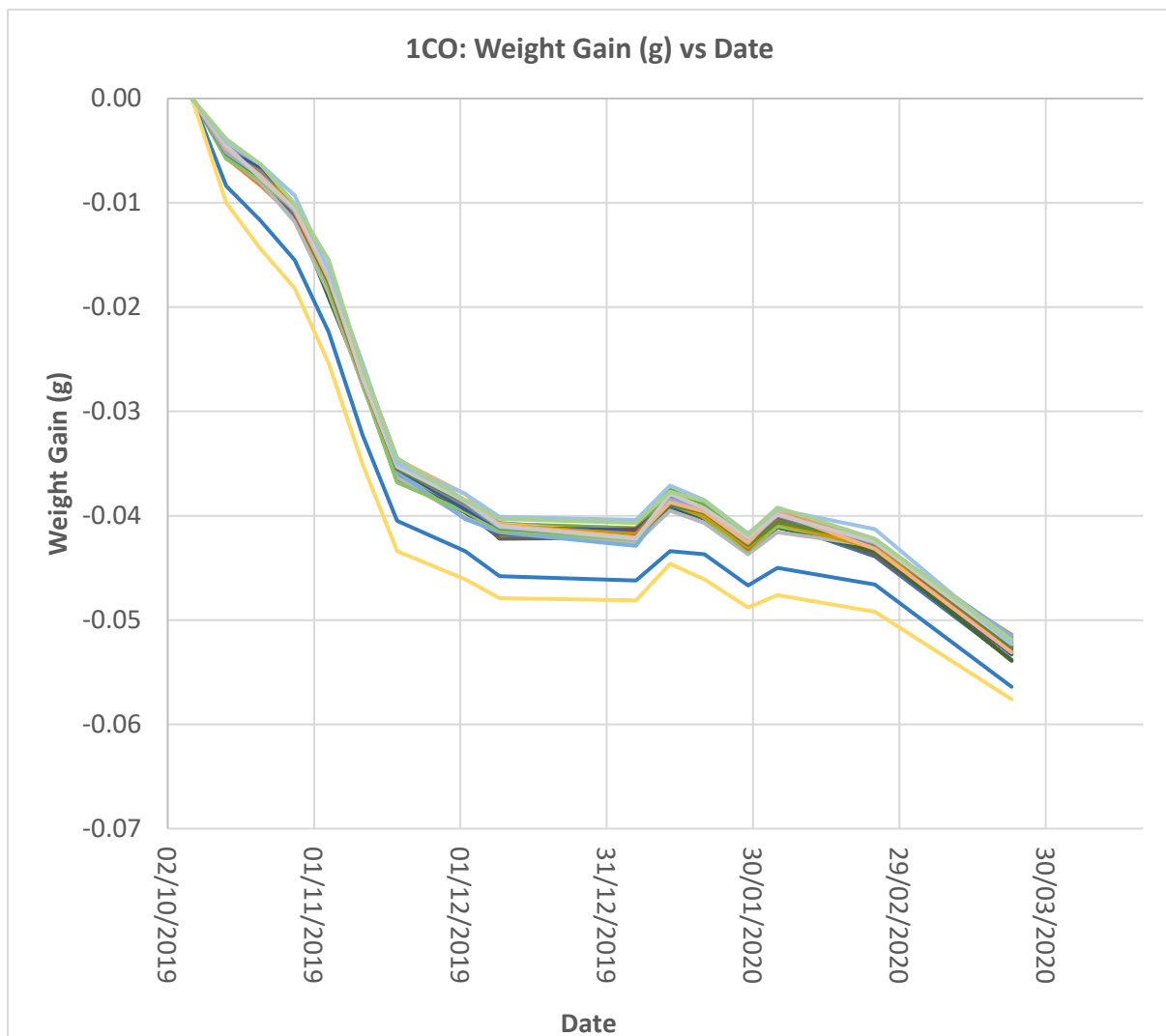
Figure 8. The humidity in the storage area dropped, causing sensors to lose water over time.
